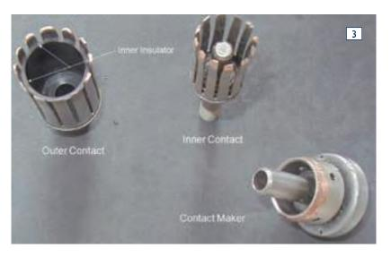
contacts. This is fragile and must be treated with great respect to avoid breakage. Pictures 2 and 3 show the contacts separated. The damage caused to the contacts is clear to see.
