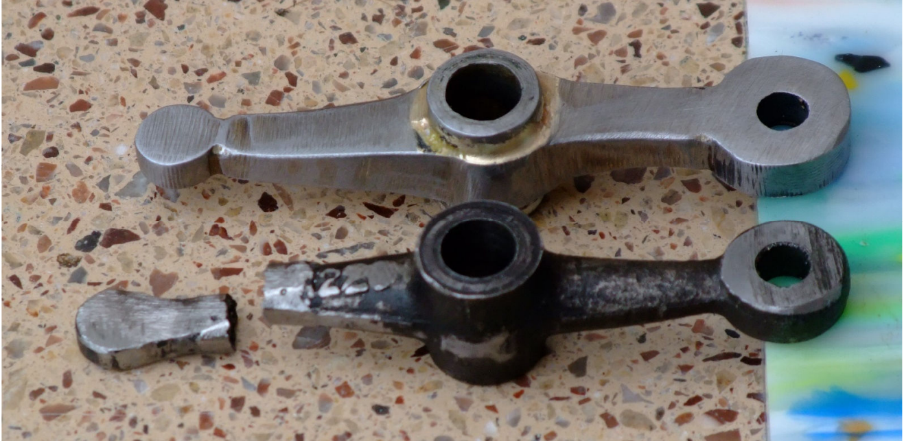
Showing broken rocker arm and roughed out new rocker arm, prior to final shaping
