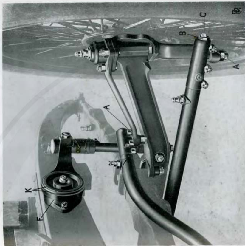
FIG. 25. CROSS STEERING TUBE AND FRONT SHOCK ABSORBER.
