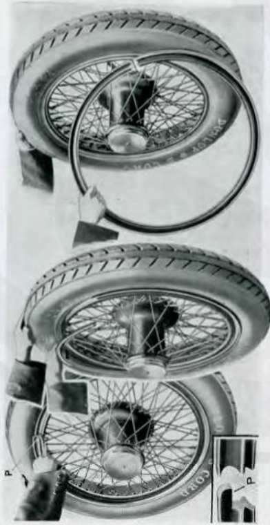
FIG. 35. REMOVING THE SIDE FLANGE.
