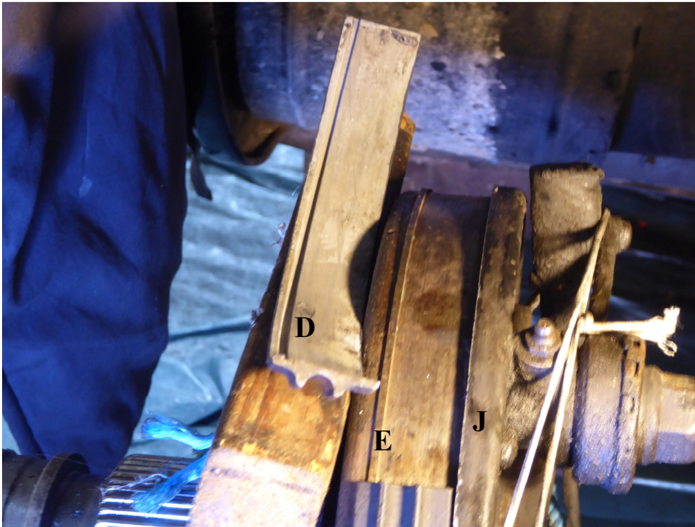
Figure 2 One of the aluminium sectors removed from the front brake shoe, showing channel in sector (D) and spigot on brake shoe (E)
