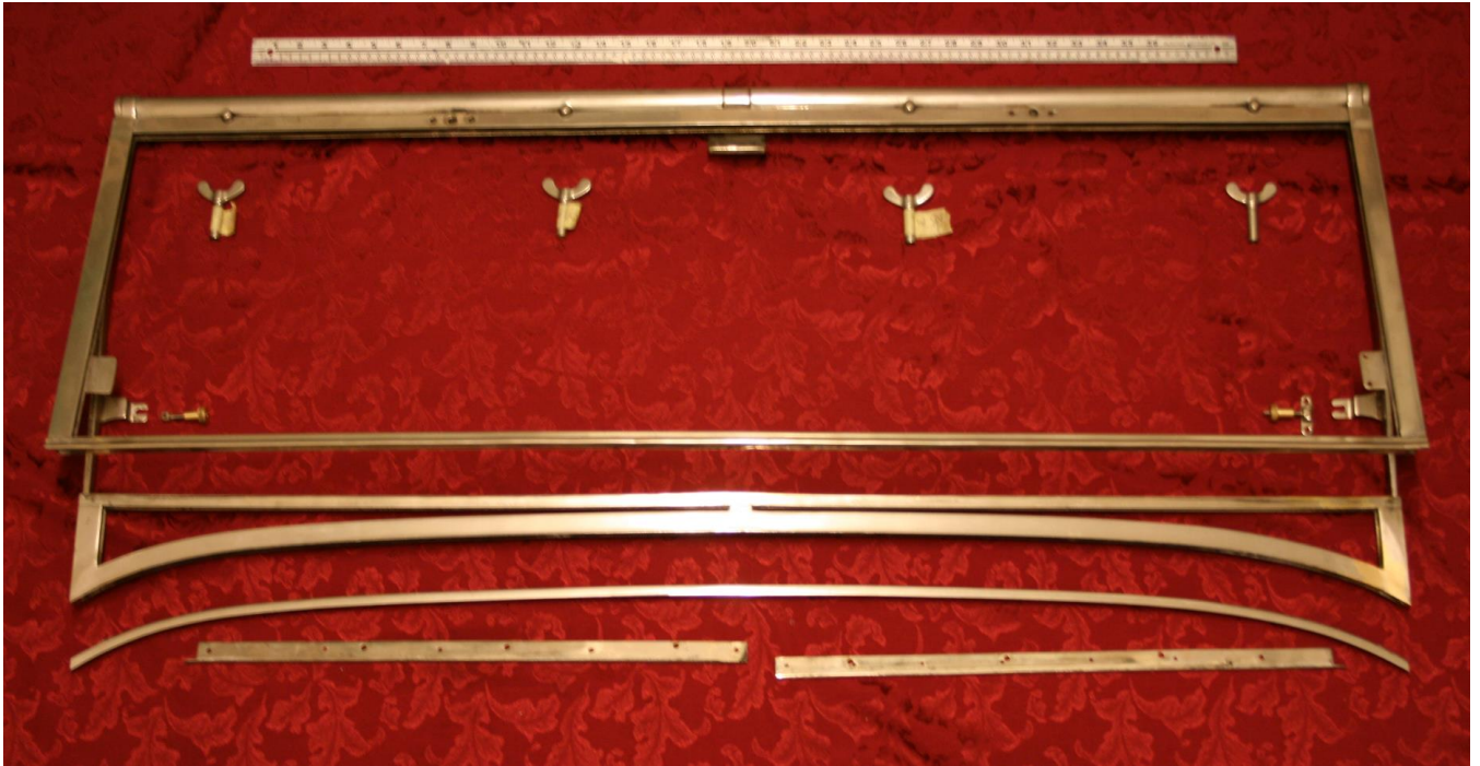
Photograph 1 Window frame, repaired and prior to dull nickel plating
