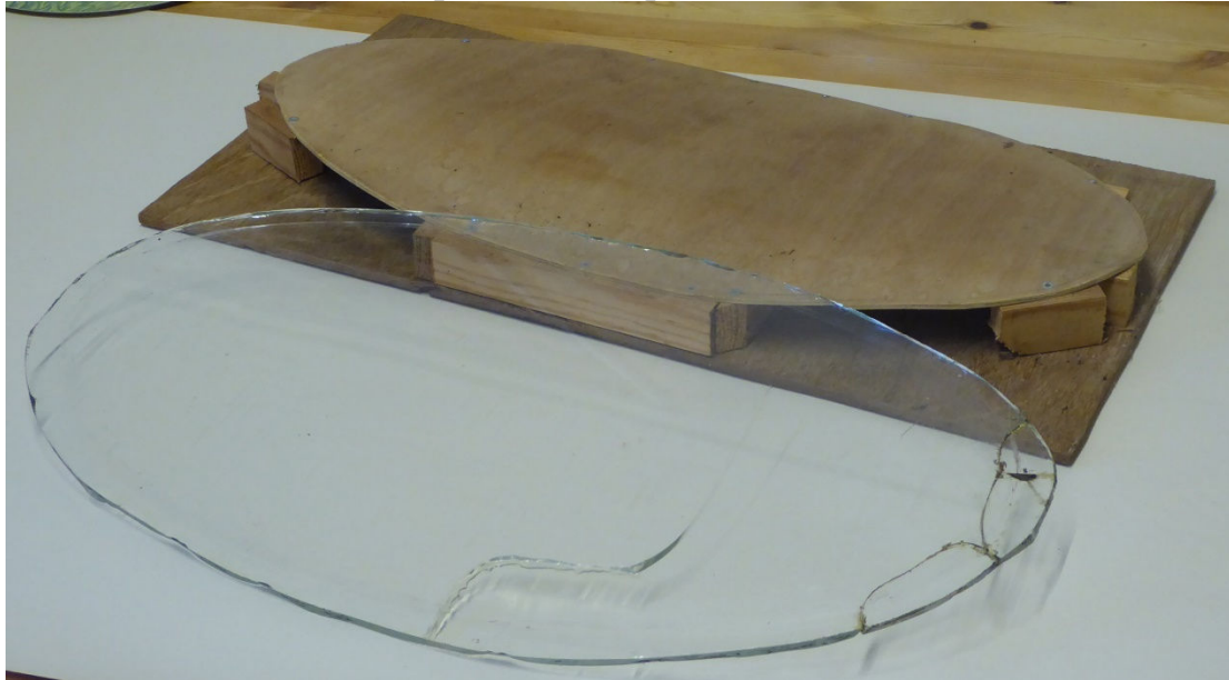
Old glass and wood former for shaping the polycarbonate
