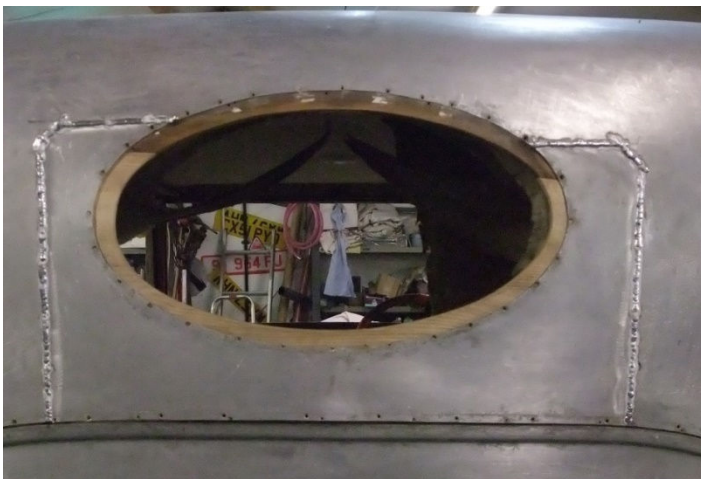
Repaired rear window frame – outer
