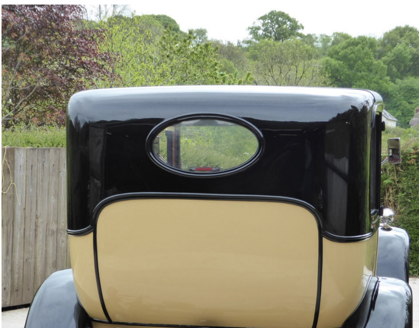
Repaired rear window frame – outer
