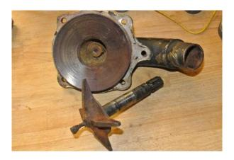
The bushings and the new hydraulic seals can be assembled on the shaft using a good helping of water pump grease. Insert the shaft into the pump, then screw on the left-hand threaded impellor.
