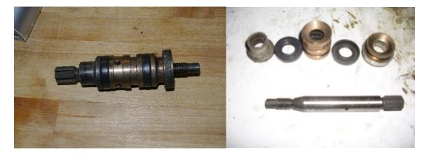
The above pictures show the new seals on and off the drive shaft. The orientation of the shaft on the first picture, should be the other way around.
