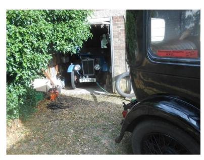
but I door. had forgotten how overgrown it would be so did not bring cutters etc. I managed to get the up and over door high enough & propped open to get the car out. As suspected the brakes were seized on. early hydraulic brakes I had fitted in 1960 had aluminium pistons in cast iron cylinders & these were always prone to seize up if the car was not used for months. The handbrake
